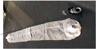
Pipe reduction and Net to control the by pass (6 m long, 0.50 m in diam, mesh size : 2 mm)
